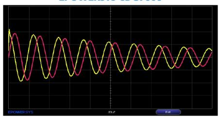
Consistent frecuency during the test. Capacitance is constant during the test  $2\mu F$
