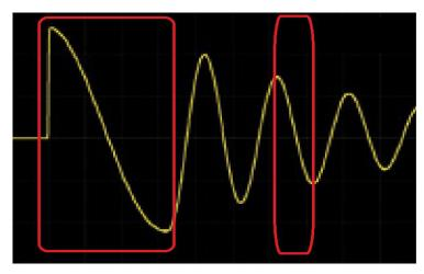
First pulse is wider than the rest of the resonance. Capacitance is reduced during the test.
